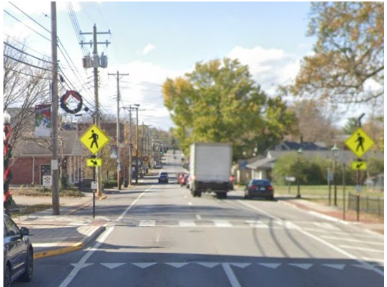
Example of midblock crossing on Midland Trail in Shelbyville, KY. Photo courtesy of Google.
